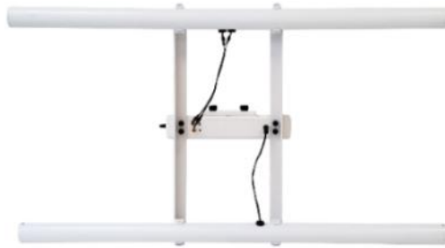
The two antenna tubes assembled and connected to the radar unit.
