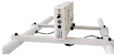
The two antenna tubes assembled and connected to the radar unit.
