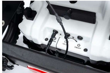
Connect the encoder cable to the EL Core antenna. If you are using a GX antenna, also use the provided adapter.
