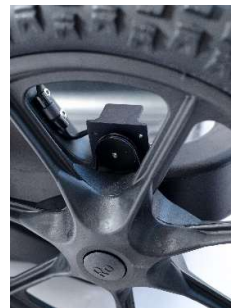
Make sure the O-ring is correctly mounted on the encoder wheel.
