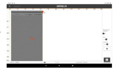
If you want to use a known object (as a pipe on a known depth) press and hold the object for a longer time period, insert the depth, the depth scale and velocity of the radargram will change accordingly.
