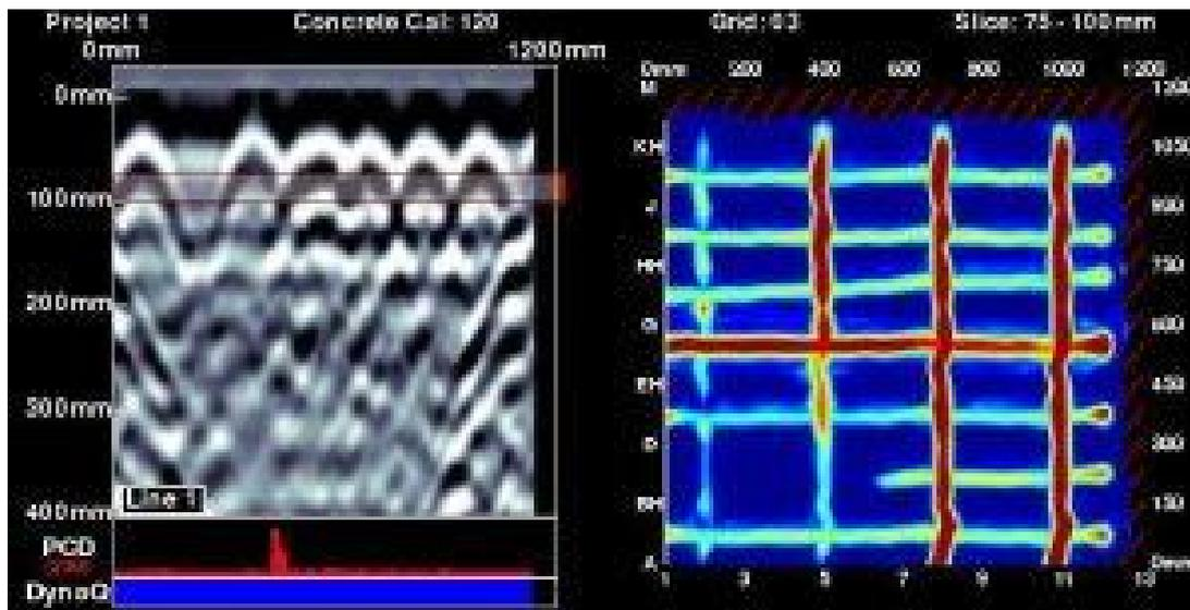
*Dan Bigman GPR produces a 2D profile of what is below the surface (left). When several 2D profiles are collected next to each other, then they can be resampled into a series of “time-slices” or “depth maps” that show embedded targets at varying depths (right).*
