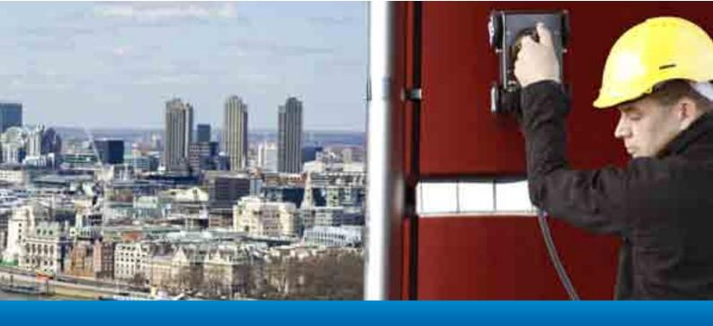
Non Destructive Testing (NDT) professionals routinely use GPR for various applications, including concrete testing. Prior to the use of high frequency (above 1 GHz) GPR transducers, x-ray methods were the primary tool for imaging structural embedment in concrete.
